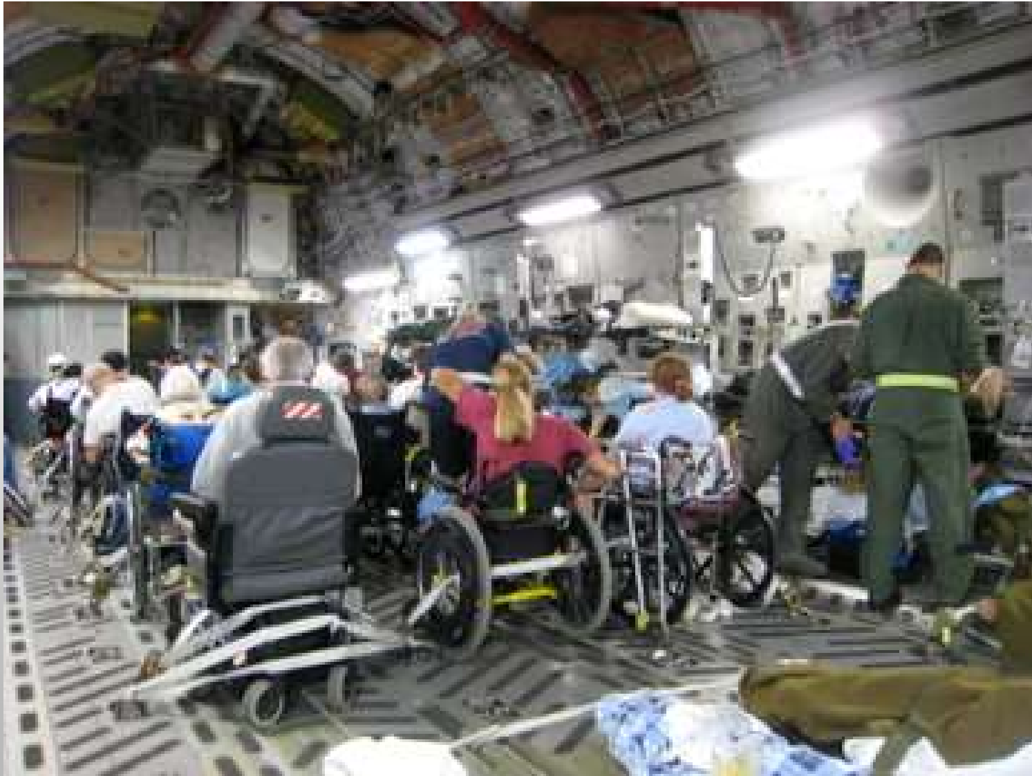
C-17 loaded with medical special needs patients. Note: wheelchairs and cots are strapped down to cargo latches.
